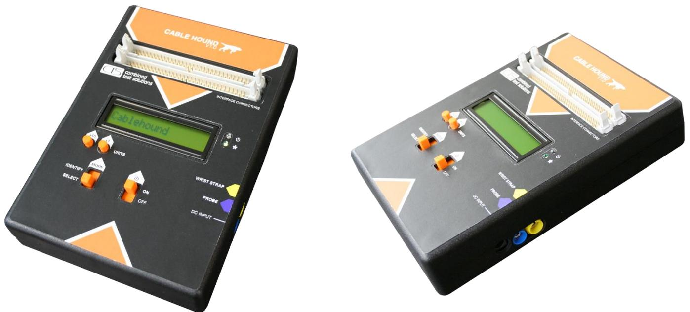
When you have cable assembly to build – perhaps a main connector, that branches out to two smaller ones, all fine pitch, expensive aerospace connectors and there's no room for error. Cablehound lets you touch a wire and it tells you what pin its connected to – so you know where to place it on the corresponding pin of the other connector. Get it right first time with the CTS Cablehound.
